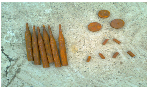
Fig.6 Specimen after tests after six months of Corrosion
