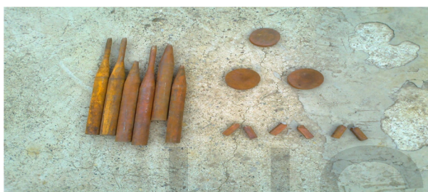
Fig.5 Specimen after tests after four months of Corrosion
